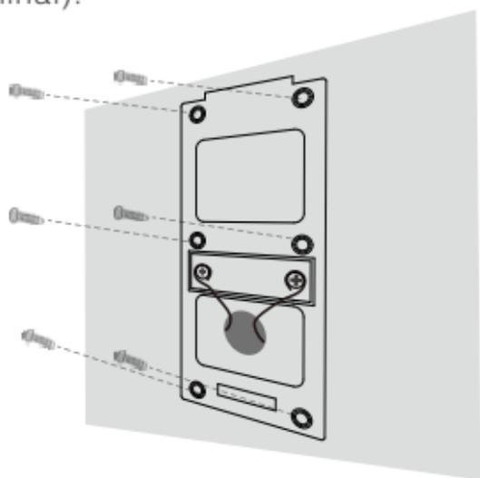
Note: When mounting on brick, concrete or stucco, use the provided screws with anchors. When mounting on wood or vinyl, drill the surface.
